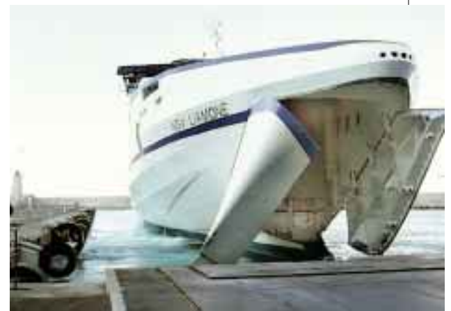
I n the Port of Nice, a simple quay construction without dedicated facilities provides high flexibility for the port, but increases the demands on the vessel.
