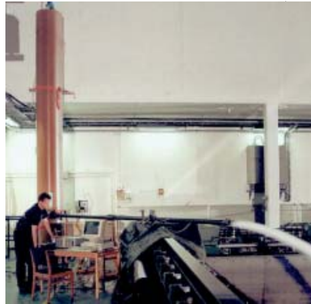
P ipe friction measurement device for surfaces with expected high increase in friction.
