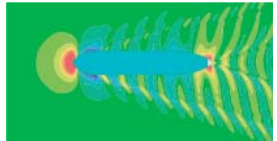
W ave and pressure contour plot showing a typical result from a hull shape optimisation using SHIPFLOW. The lower half of the picture shows the original hull design of a VLCC and the upper half shows the improved design.
