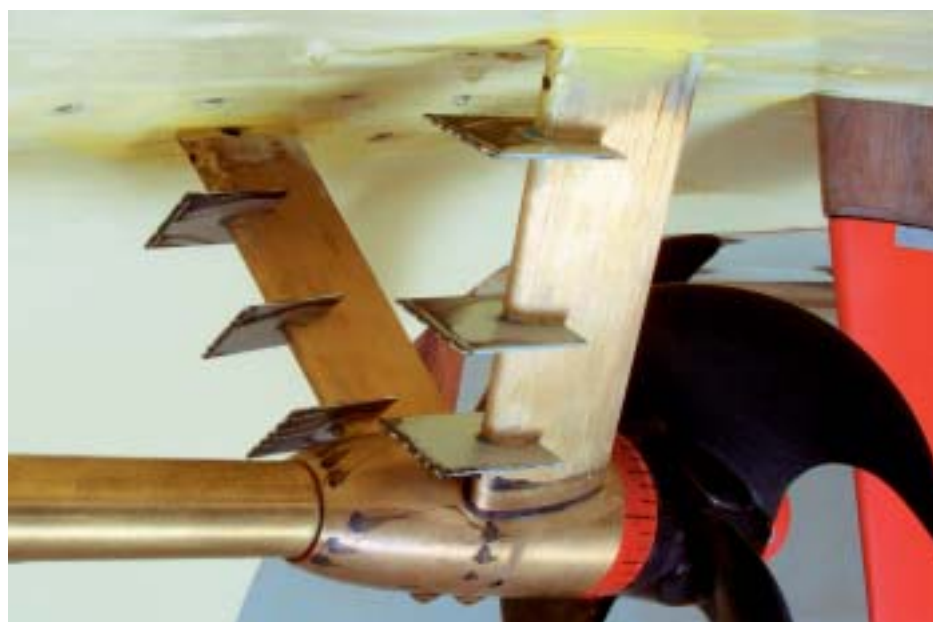
P otentially erosive rudder cavitation in model scale. 3° rudder angle is applied.
