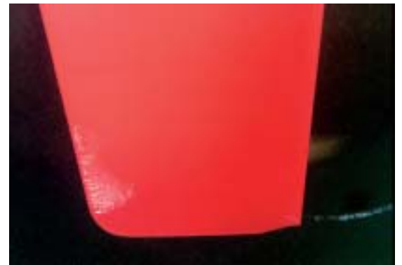
P otentially erosive rudder cavitation in model scale. 3° rudder angle is applied.
