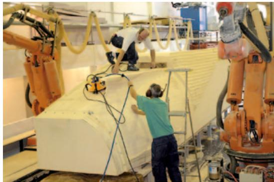
Divinycell core. Bonding the load-carrying structure together with the outer hull and construction of deck hatches and superstructure.
