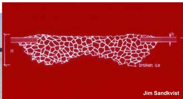
The test channel of approximately 1/2 nm in the port of Luleå. Inserted is a general example of channel profile. Channel edge depths up to several meters were measured.
