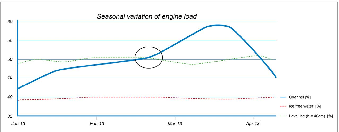
Engine load for each channel passage and corresponding reference tests in level ice and ice free water. Note where channel load crosses the level ice load, hence a parallel channel favourable.
