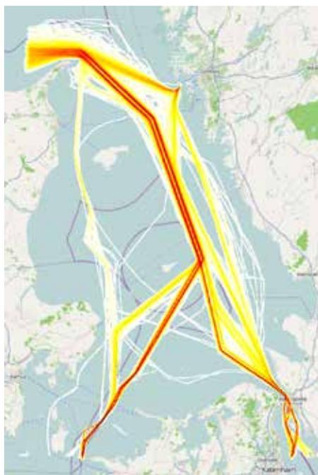
*Density plot for the current main transit traffic through the Kattegat. Carried out with the IWRAP risk assessment tool, based on Helcom's AIS data for January 2012. (Recalculated to one year.)*
