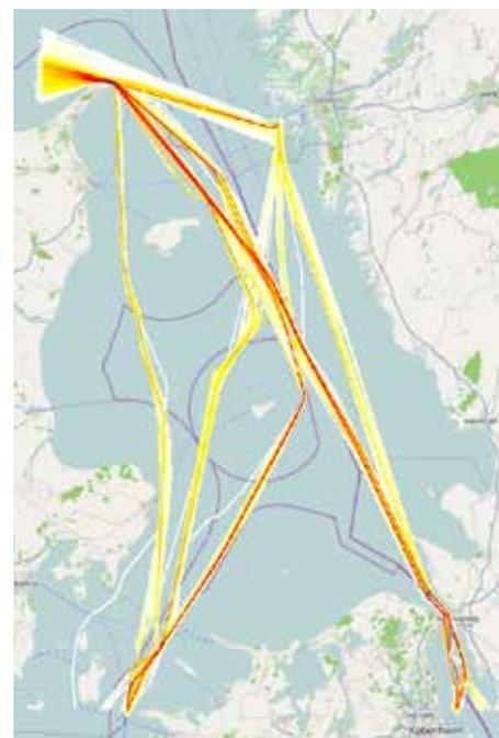
*Density plot for the optimised routes. Carried out with the IWRAP risk assessment tool, based on SSPA's simulated AIS traffic data from optimised routes. (Recalculated to one year.)*
