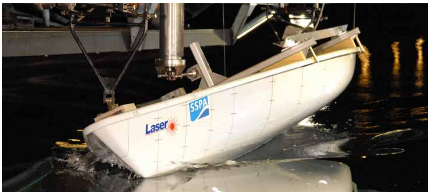
*Optimum heel for downwind sailing in the speed range of 3 to 8 knots.*
