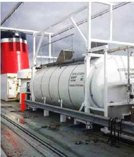
*Methanol is a liquid at ambient temperature and pressure and was stored in a tank container for the SPIRETH project.*
