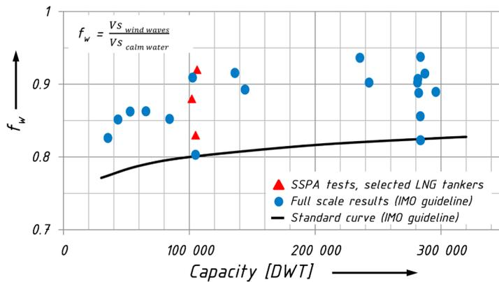
$f_w$  factors for tankers. Ship-specific model test (red triangles) can give a much more favourable  $f_w$ -value than the simplified standard curve (black line).
