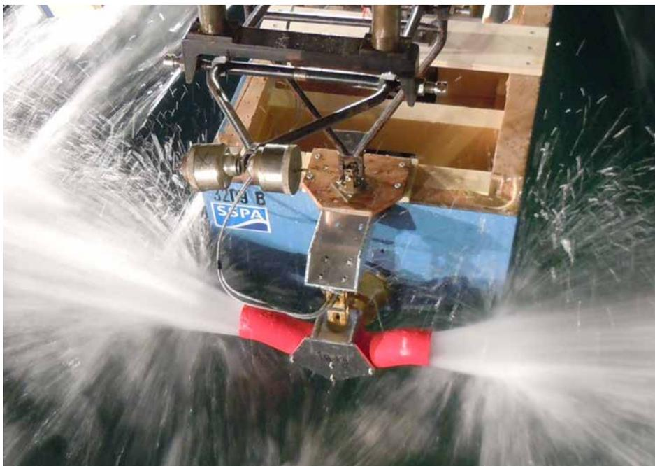
*T-junction during model test at high speed.*
