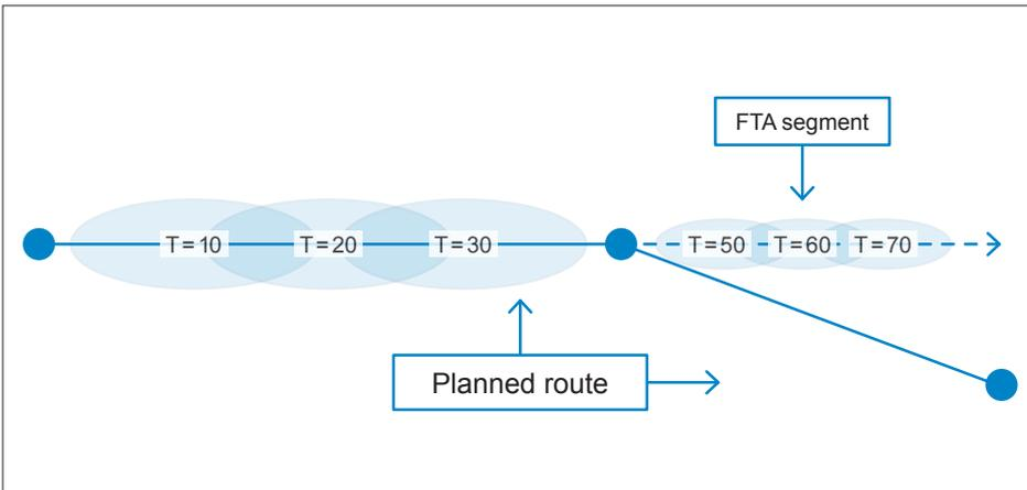
Safety ellipse travelling on the route and ellipse with vessel length and beam on the FTA segment.
