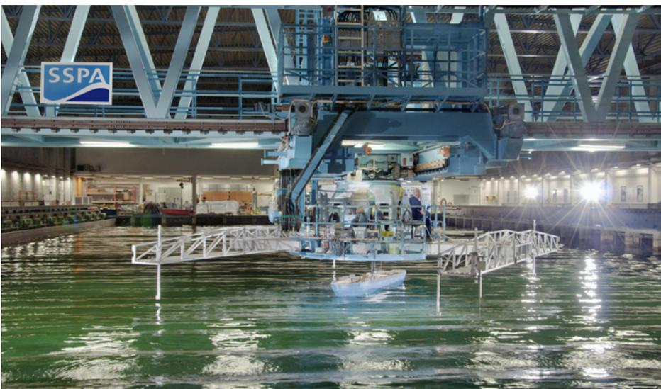
*SSPA Marine Dynamics Laboratory – the useful tool for verifying seakeeping and manoeuvring performance. The free sailing model will ensure correct ship behaviour. Photo: Anders Mikaelsson.*
