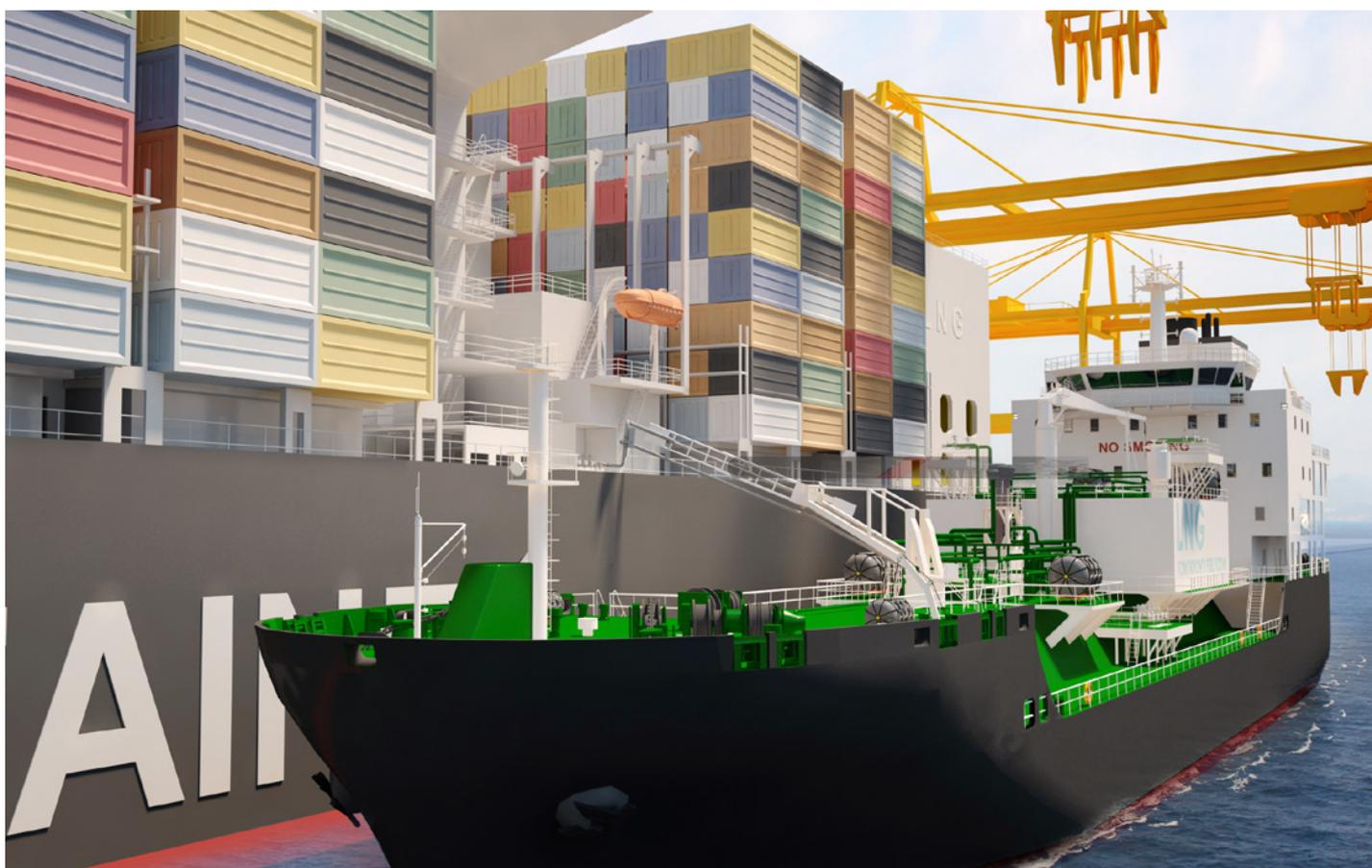
*The STX 6500 LNG bunker vessel is under construction in South Korea. LBVs are short in length in order to be able to manoeuvre in port, and this means they will also be fairly wide in beam to be able to carry the desired amount of LNG. Finding the best compromise between cargo capacity, propulsion efficiency and manoeuvrability is the key to success. Courtesy of STX Offshore & Shipbuilding.*
