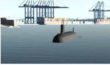
A submarine in a simulator environment. The crew can practise repeat manoeuvres and practise operations which are not easy to perform on a real submarine.
