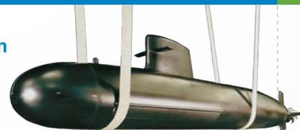
*Model of the IZAR P650 tested at SSPA. The same model was used in all SSPA facilities.*
