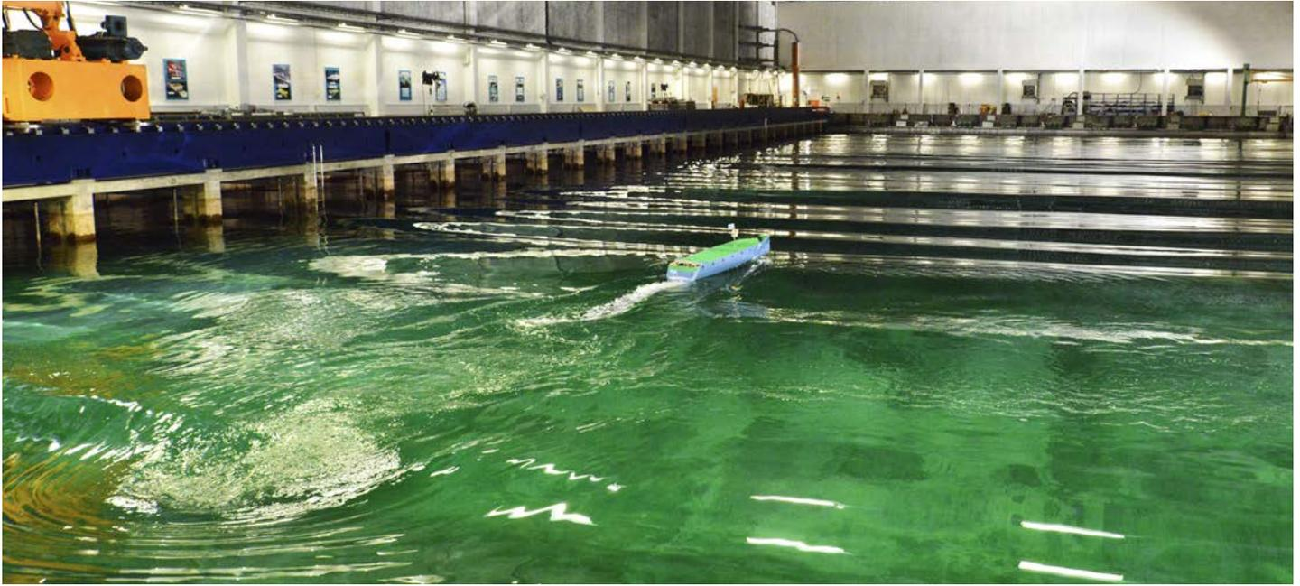
Photo of the 24 m motor yacht tested in SSPA's large seakeeping and manoeuvring basin MDL (Maritime Dynamics Laboratory). Photo: Anders Mikaelsson.
