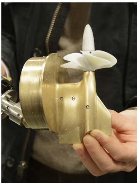
*One of the two driving units / thrusters of pulling propeller type. Photo: Anders Mikaelsson.*
