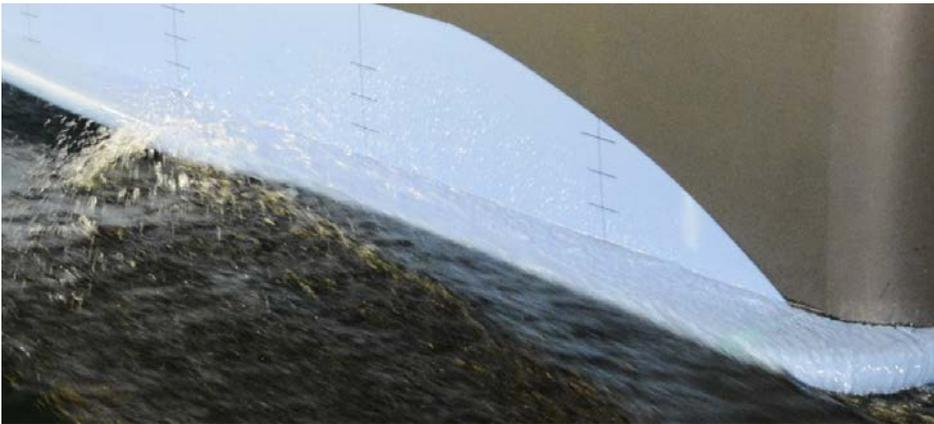
This observation during towing tests might lead to another design of the platform. Photo: SSPA.
