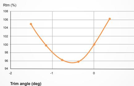
The Y-axis is showing total resistance for each load case (trim at rest) in % of the resistance for the vessel loaded to even keel.
