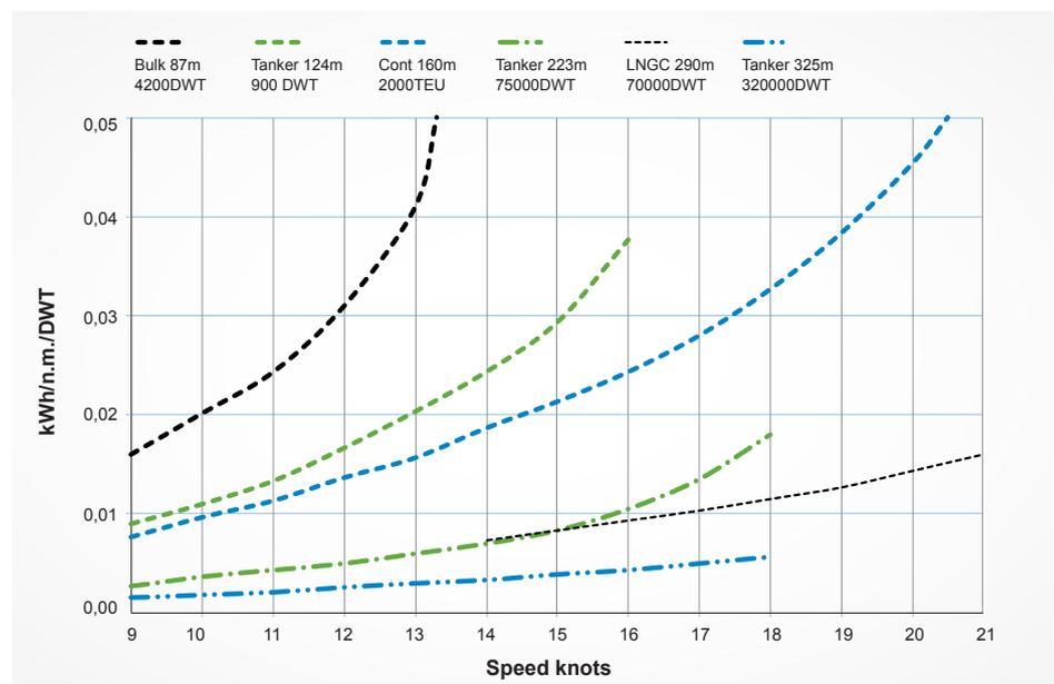
Energy consumption per tonne-km for a few examples of ships. Figure: SSPA.
