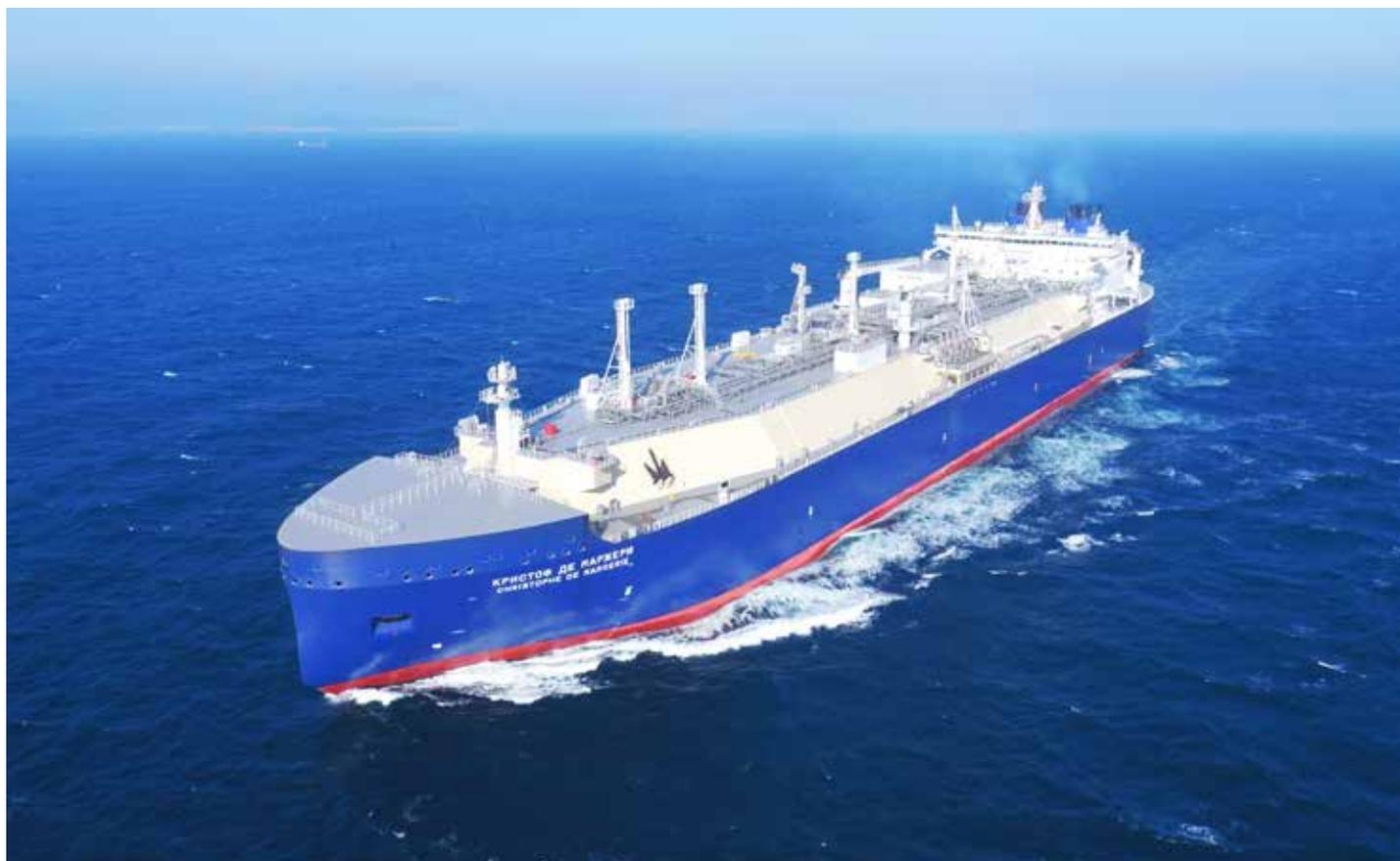
This 170,000m<sup>3</sup> LNG carrier with ice-class Arc 7 was built for Sovcomflot for a charter to Yamal LNG for 28 years. Courtesy of DSME.
