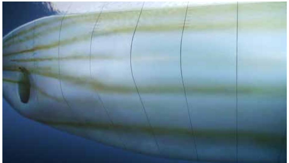
*Coffee test: the test method uses stained water, which is let out through the hull in certain representative locations. This method is quick and effective, and shows how and where sensitive equipment can be placed in order to minimise the disturbance from unwanted flow fields.*
