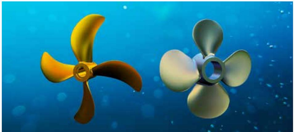
*These two propellers are both designed for 170,000 m<sup>3</sup> LNG carriers with a design speed of 19.5 knots at design draught. The same type of vessel but with totally different operational profiles. One is designed and optimised for open water, the other for operation in ice. The difference in installed power and thus the fuel cost for the two cases is substantial. A correctly balanced solution with regards to operational profile saves money.*
