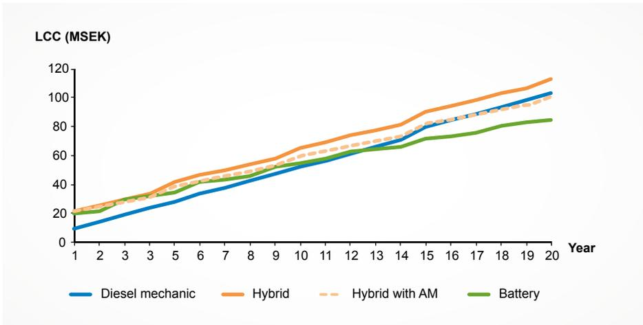
The accumulated LCC for four different concepts of propulsion.
