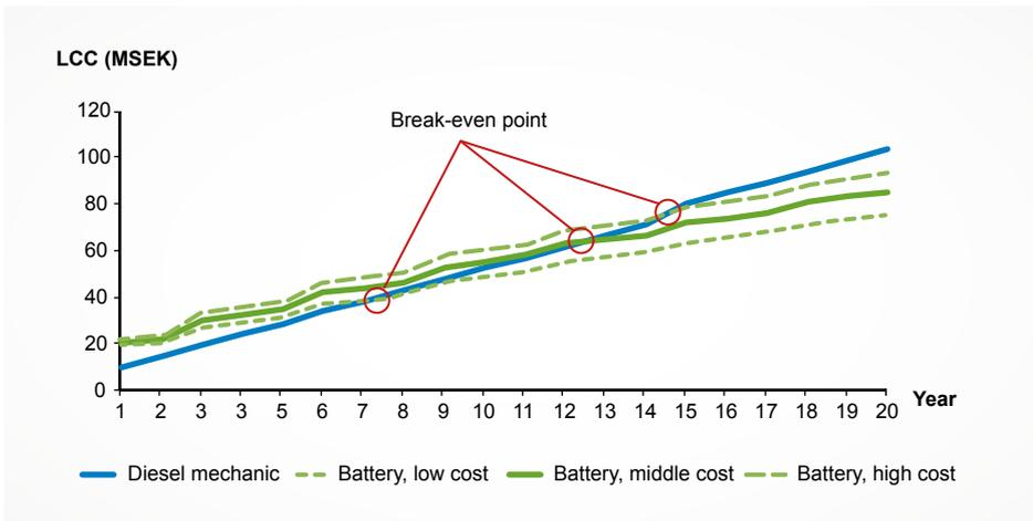
The accumulated LCC for the “Diesel mechanic” and “Battery” concepts. The LCC for the battery concept is given for three different scenarios: low, middle and high battery cost.
