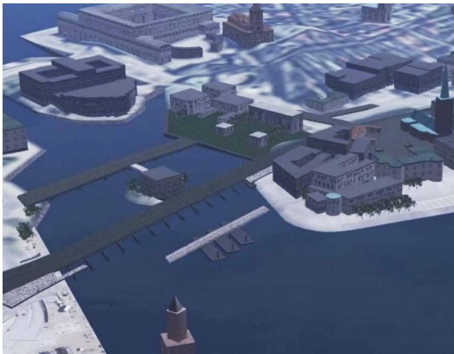
*In these simulations, it was assumed that the barge will be using winches connected to the shoreline and anchors for positioning. The tugs will be disconnected from the barges before this critical section. Illustration: SSPA*
