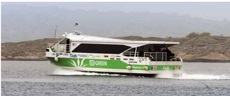
At SSPA, increased activity within the area of battery and hybrid propulsion can be seen in an increasing number of projects within this area. One example is the fast, air-supported commuter ferry “Airi El” in the project BB GREEN. Photo: Anders Mikaelsson, SSPA.
