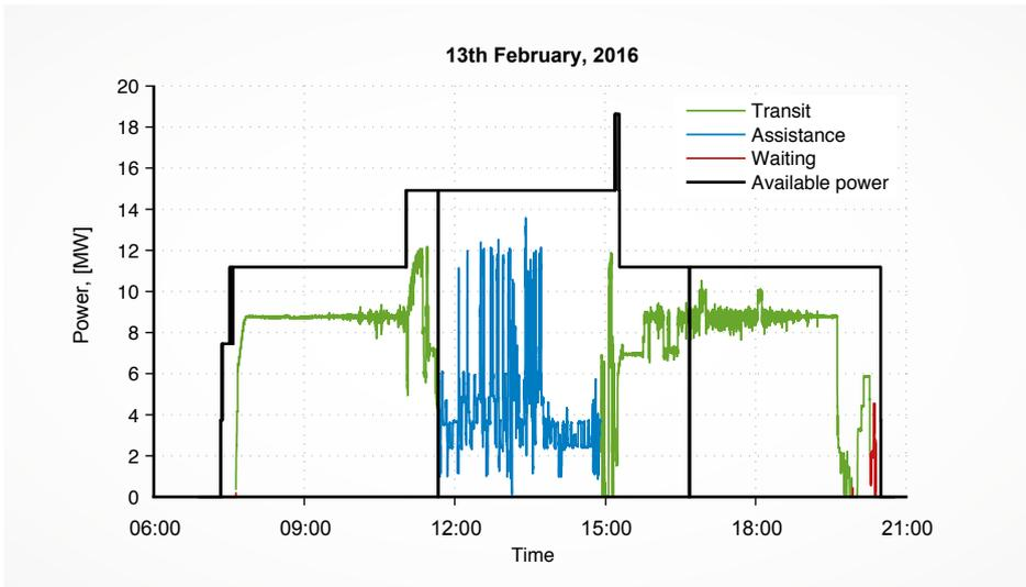
The figure shows total propulsion power along with the available power for an icebreaker during a typical icebreaking mission. Illustration: SSPA.
