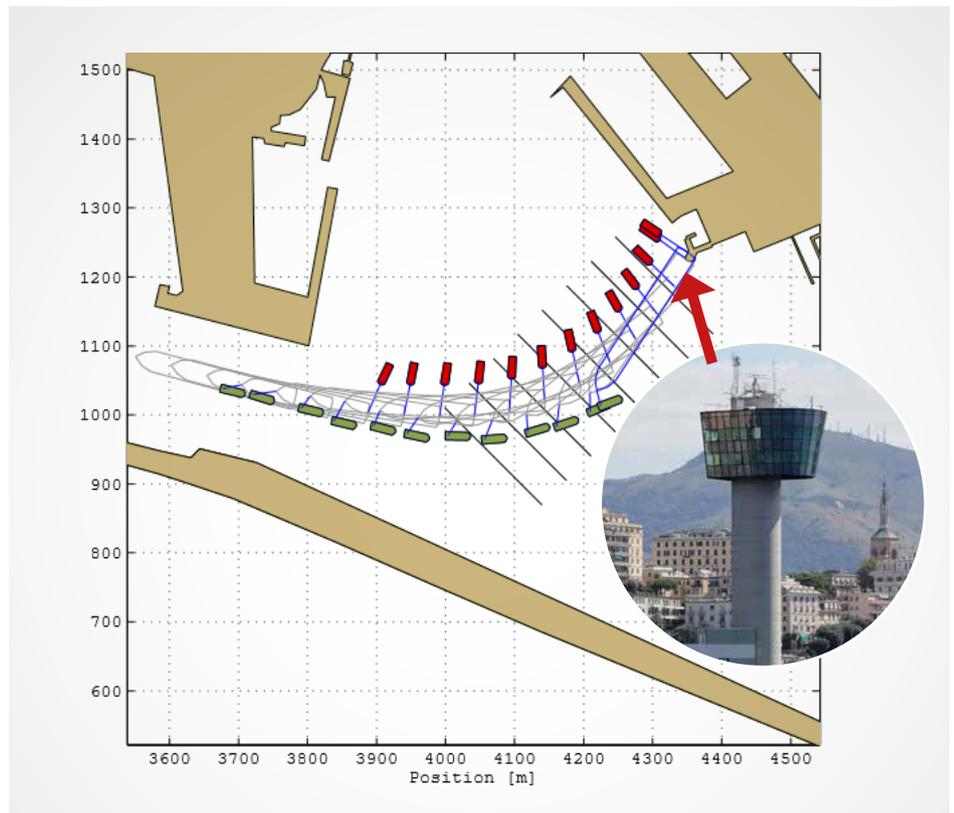
The reconstructed track of the Jolly Nero and the tug prior to the collision with the control tower. The stern and bow tug is indicated in red and green respectively. Illustration: SSPA.
