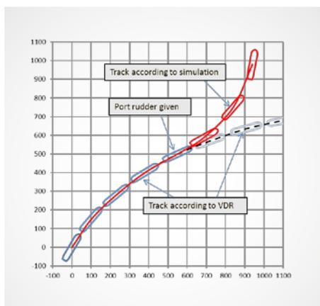
VDR data is used initially. When a manoeuvring device is used, the system switches to simulation mode. Figure: SSPA.
