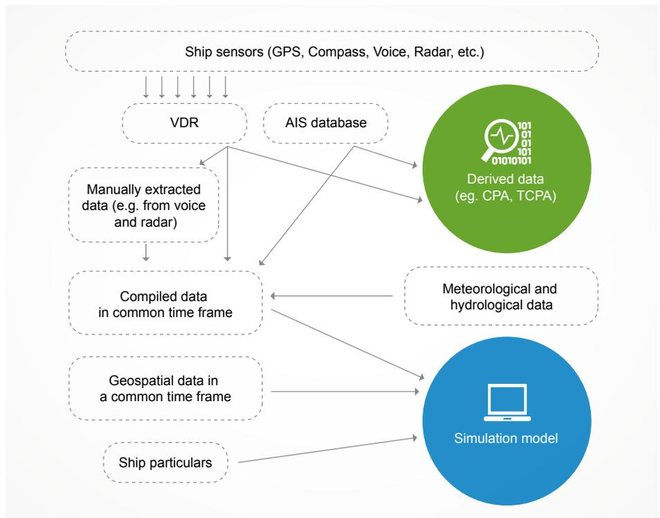
Utilisation of data sources in simulations for the various sources that form the basis of the simulation system. Illustration: SSPA.
