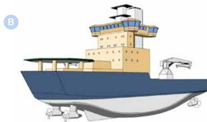
Concept A consists of twin rudder and shaft propellers in the aft and twin shaft propellers in the fore, while concept B uses POD propulsion (integrated electric motor/propeller unit mounted on the same shaft), two in the fore and two in the aft.
