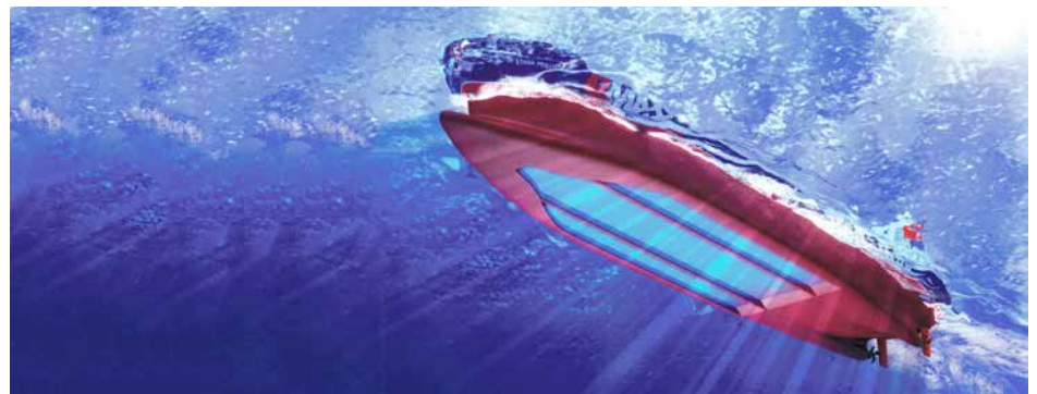
SSPA investigated different designs for the project P-MAX air to minimise the resistance of the 182 m tanker. Photo: Courtesy of STENA AB. Read more at www.sspa.se
