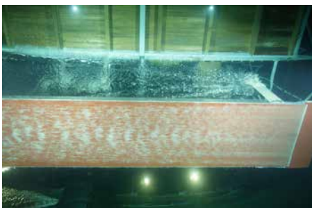
Through the EU project SMOOTH, SSPA has tested a concept on flat plates and measured the effect of different parameters on minimising the friction. Read more at www.smooth-ships.eu
