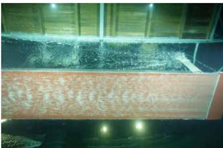
Through the EU project SMOOTH, SSPA has tested a concept on flat plates and measured the effect of different parameters on minimising the friction. Read more at [www.smooth-ships.eu](http://www.smooth-ships.eu)
