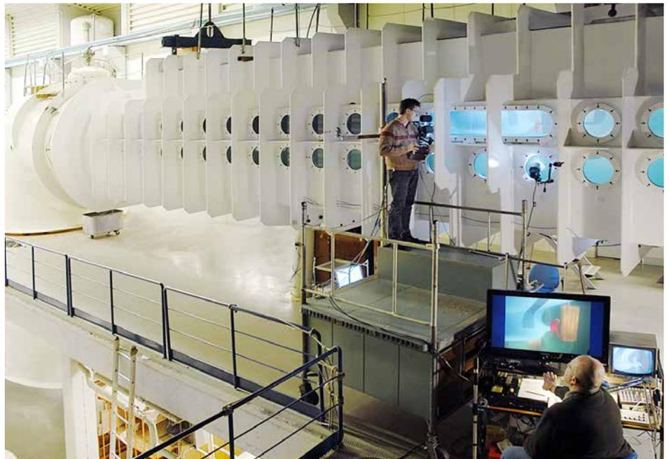
*Has this propeller risk of cavitation erosion damage? Ongoing tests on a propeller in our Cavitation tunnel. Photo: Anders Mikaelsson, SSPA.*
