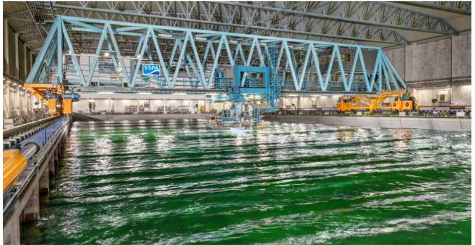
Ongoing research to increase knowledge of a ship's added resistance in waves. SSPA is now conducting a research project to increase the accuracy and efficiency of detecting added resistance in waves experimentally and numerically. Photo: Anders Mikaelsson, SSPA.
