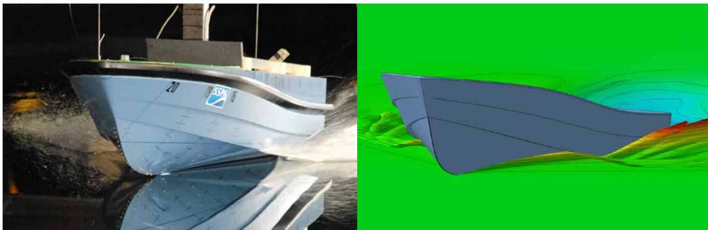
Analysing the energy efficiency of the hull on RS 158 Idar Ulstein using EFD, (Experimental Fluid Dynamics) and CFD (Computational Fluid Dynamics).
