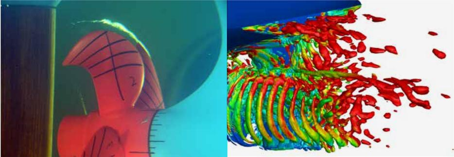
Measuring the propeller efficiency and cavitation erosion, examples of evaluation using EFD and CFD.
