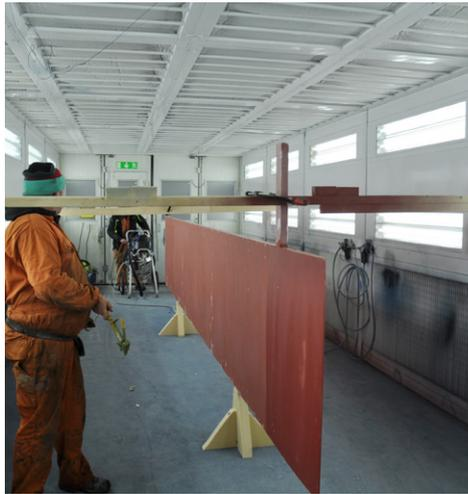
*Antifouling coating applied with same procedure as on a full-scale vessel.*
