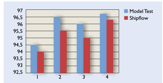
**E**nergy gain predicted by CFD (left) and model test (right) for different PSS configurations.
