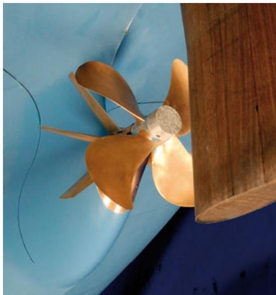
**P** SS mounted on ship model for testing.
