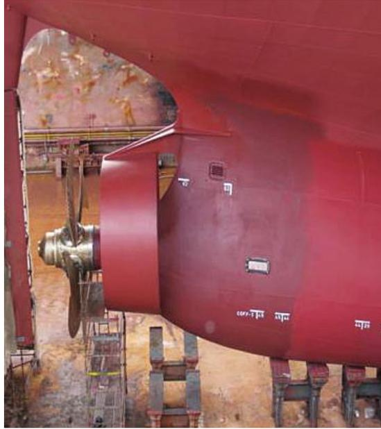
*Installation of a Mewis Duct® on MR tanker "Tambourine" in November 2009.*
